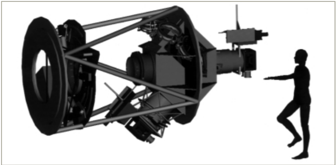
Fig. 1. This is a model of the Inamori Magellan Areal Camera and Spectrograph (IMACS) to be mounted on the Magellan I telescope. When complete, this wide-field instrument will be used in high-redshift studies of the universe.
